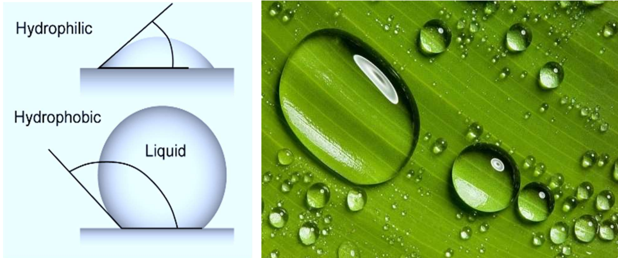
Figure 3: Illustration 1 of difference in surface energy of substrate (non-polar to polar) to water droplets (polar). Hydrophobic conformal coatings may have dramatic difference in moisture permeability. It is critical that hydrophobic conformal coatings be coupled with high moisture barrier (low moisture permeability) to be effective in protecting printed circuit boards.
