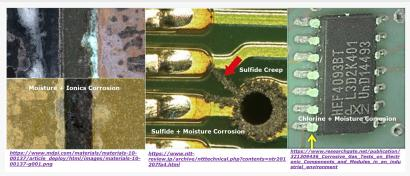
Corrosions in exposed based metal traces such as copper and nickel-plated contacts, solder interconnections, plated through vias happens when there is a condensed moisture laden with dissolved salts and ionic impurities, corrosive gases such as H2S, CO2,
