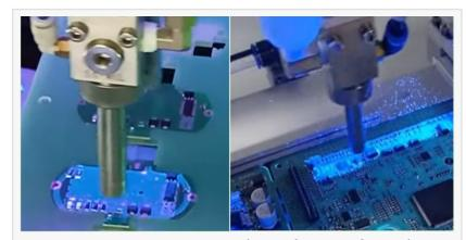
MOISTSEAL™ CC7650 is a solvent-free conformal coating that can be applied with traditional spray, dip, and brush coating in a common electronic manufacturing environment without excessive ventilation provision. It can also be applied in the field for fiel
