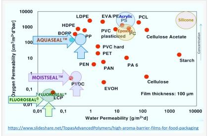
MOISTSEAL™ CC7650 has a more than 100 times higher moisture and corrosive gases barrier than traditional acrylic conformal coatings. Its solvent-free, waterborne, and fast drying solution provides the ease of field applicability and more manufacturability
